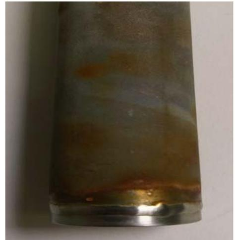
Figure 3. Rust starts due to improper care.
