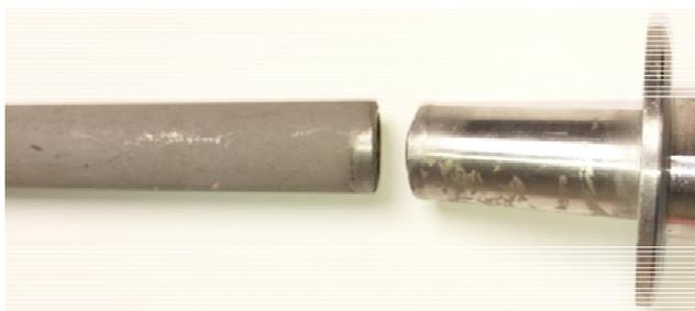
Figure 4. Carb stone treated carelessly with other fittings.
