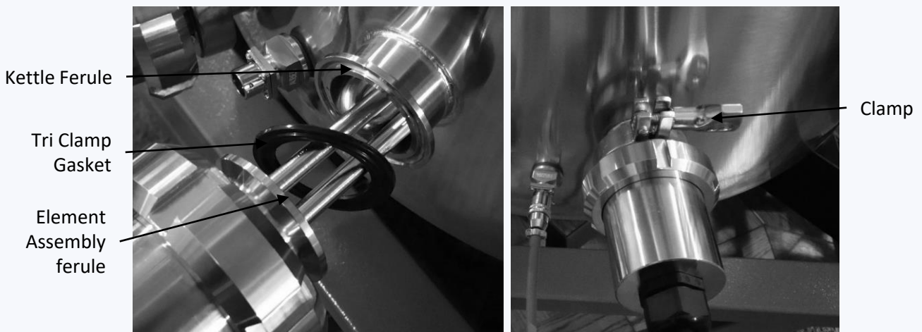
Installing Element
