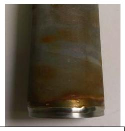
Figure 3. Rust starts due to improper care.
